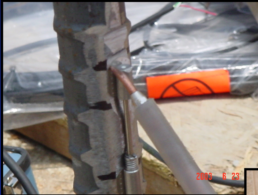
Spot welding strain gauge
