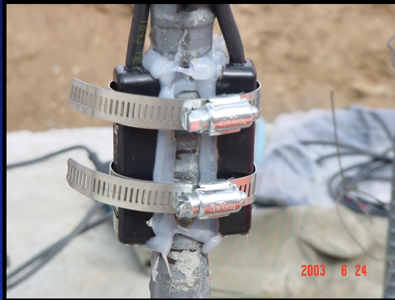
Installed strain gauge (typical)
